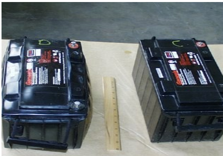
Example of a swollen, failing battery.
