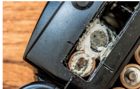
Example of household battery corrosion.
